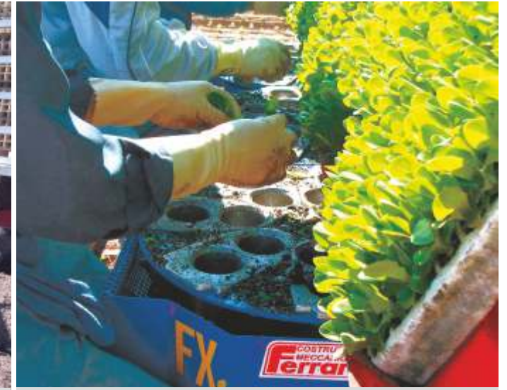
DISTRIBUTORE INTERMITTENTE | STEP BY STEP CAROUSEL BARILLET INTERMITTENT | INTERMITTIERENDER VERTEILER DISTRIBUIDOR INTERMITENTE
